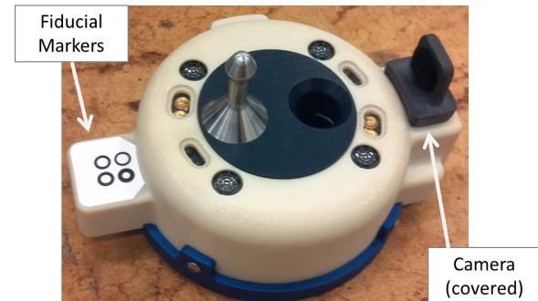
Figure 2: The SPHERES Universal Docking Ports can be used for sensing and estimation by virtue of an onboard camera.
