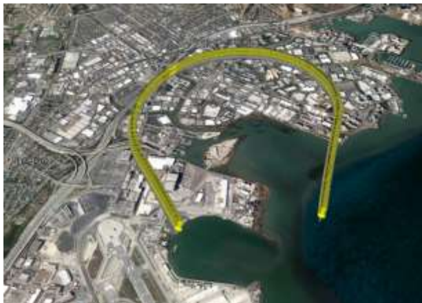
Steady level turn executed by the aircraft
